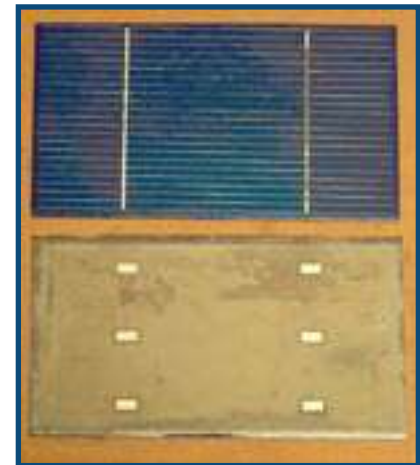
Above, older style cells, with solder covering the backs; below, newer cell with six solder spots on the back.
