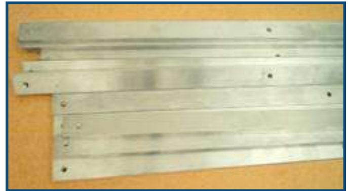
Side bars, drilled and tapped.
