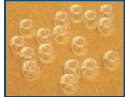
Plastic beads are used as spacers to keep the Plexiglas cover from touching the cells
