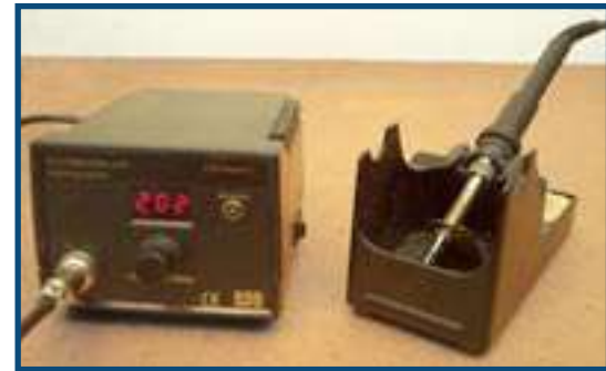
Soldering iron with digital readout and temperature control
