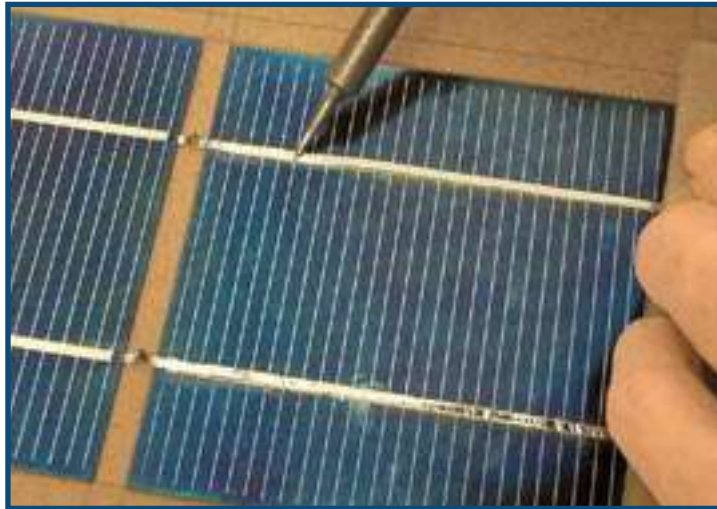
Solder the tab ribbon to the face of the next cell
